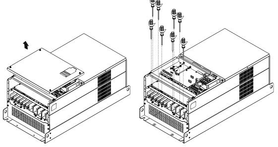
Install the conduit box by fastening all the screws shown in the following figure. M5 Screw torque: 24~26kg-cm (20.8~22.6lb-in) M8 Screw torque: 100~120kg-cm (86.7~104.1lb-in)
