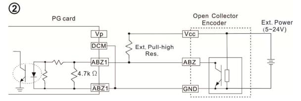
PG2 Wiring Diagram
