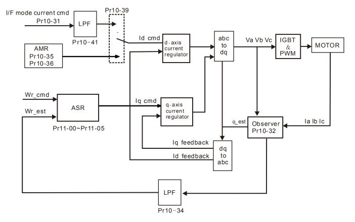
When 00-10=0, and set Pr.00-11 to 7, IPM FOC sensorless control diagram is shown as follows:
