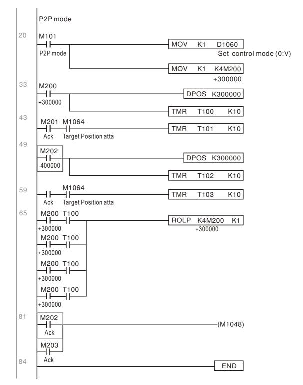
If homing is not needed in an application, the first and second parts can be skipped. However, the M1040 condition from Part 1 must be included, and the writing method in Part 1 involve the use of X2 to achieve direct access. In addition, when M101 is used at the beginning of Part 3 to set the control mode, it can be rewritten as M1002, which will put the PLC immediately into the position mode when it starts running.
