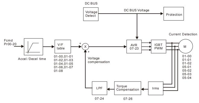
When 00-10=0, and set Pr.00-11 to 1, the V/F control + encoder diagram is shown as follows.
