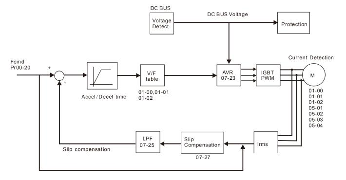
When 00-10=0, and set Pr.00-11 to 3, the IM FOCPG control diagram is shown as follows.
