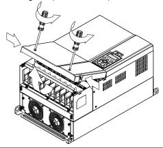
2. Remove the 5 screws shown in the following figure. Screw torque:24~26kg-cm (20.8~22.6lb-in)
