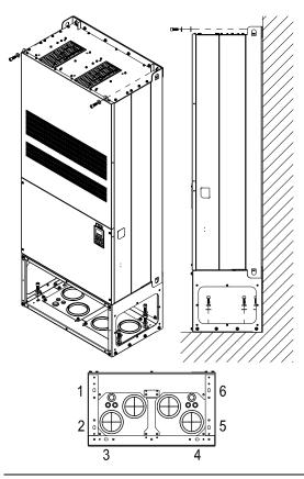
Secure the drive from the internal.
