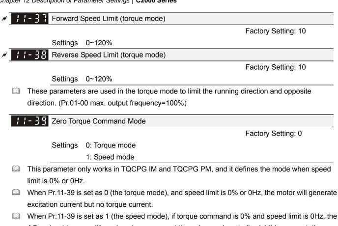
AC motor drive can still produce torque current through speed controller (at this moment, the torque limit is Pr06-12) and the control mode will change from TQCPG to FOCPG mode. The motor will have a holding torque. If the speed command is not 0, motor drive will change to be 0.
