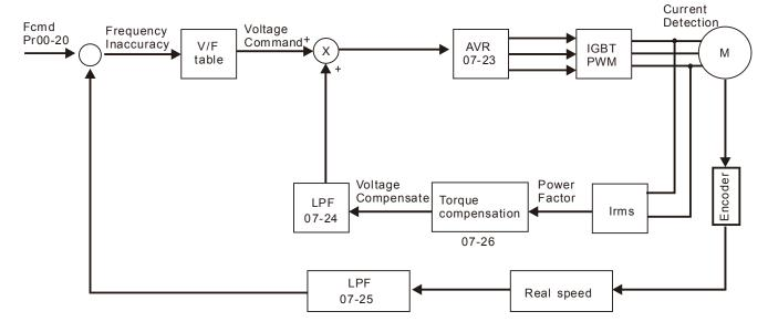
When 00-10=0, and set Pr.00-11 to 2, the sensorless vector control diagram is shown as follows.
