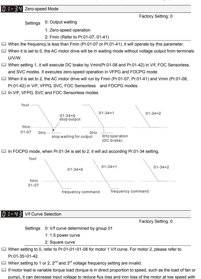
low load torque to raise the entire efficiency.
