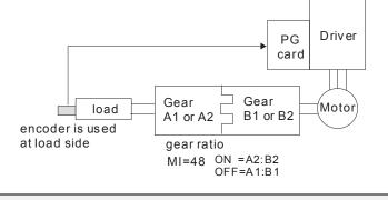
**III - III** Treatment for Encoder/ Speed Observer Feedback Fault
