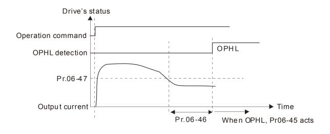
Status 2 : Motor drive is in stop; Pr06-48=0 ; Pr07-02≠0 After motor drive starts, DC brake will be applied in accord to Pr07-01 and Pr07-02. During this period, OPHL detection will not be conducted. After DC brake, motor drive starts to run, and conducts the OPHL protection as mentioned in status 1.
