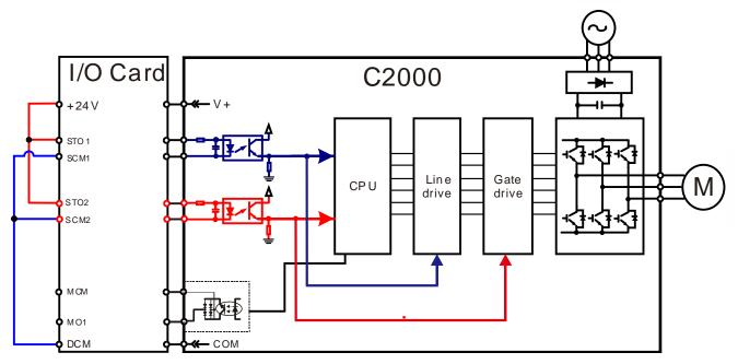
20-3-3 The control loop wiring diagram:
