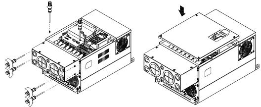
3. Fasten the 4 screws shown in the following figure. Screw torque:12~15kg-cm (10.4~13lb-in) \_
