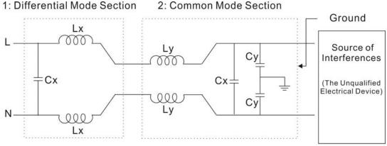
A filter is composed of a Differential Mode section (to eliminate noise below 150kHz) and a Common Mode section (to eliminate noise above 150kHz). For high-frequency noise, the inductor acts as a high impedance to form an open circuit and the capacitor acts as a low impedance to form a short circuit. Proper design and dimensioning of inductors and capacitors give a resonant circuit to absorb harmonic currents. Capacitor Cy is earthed to lead the harmonic currents to the ground.
