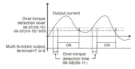
When Pr06-06 or Pr06-09 is set to 2 or 4, the motor drive will have the ot1/ot2 fault after Over Torque Detection. Then the motor drive stop running until it is manually reset.
