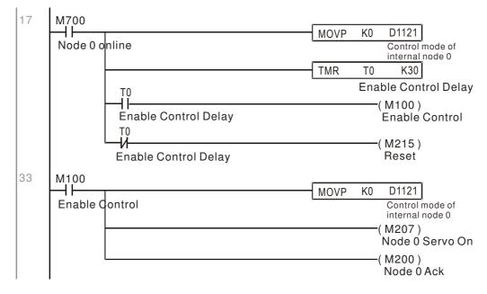
It is required slave station 1 maintain forward rotation at 30.00Hz for 1 sec., and maintain reverse rotation at 60.00 Hz for 1 sec., and repeat this cycle continuously.
