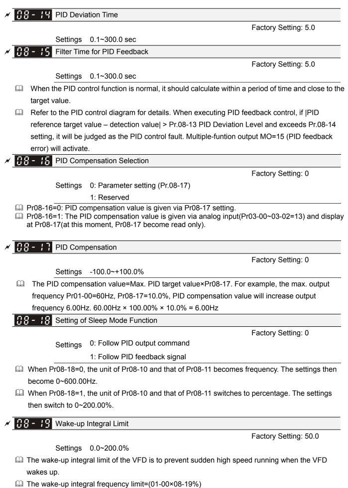
Depict of the Pr08-19 is used to reduce the reaction time from sleep to wake-up.
