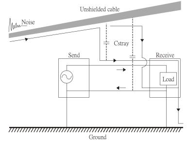
4. The common-mode noise of an unshielded power cable is transmitted to the ground via the stray capacitance. Since both shielded wire and unshielded wire are connected to a common ground, other systems can be interfered with by the common-mode noise that is transmitted from the ground back to the system via the shield. See Figure 4.
