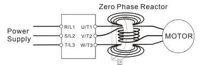
2. Place all wires through the middle of four zero-phase reactors without winding.
