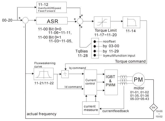
When 00-10=0, and set Pr.00-11 to 5, FOC sensorless (IM) control diagram is shown as follows.
