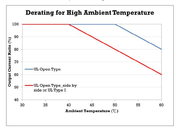
Advanced control Ambient temperature derating curve
