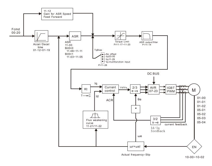
When 00-10=0, and set Pr.00-11 to 4, the PM FOCPG control diagram is shown as follows.
