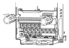
2. Remove the control board by pulling it out for a distance 6~8 cm (as 1 in the figure) then lift the control board upward(as 2 in the figure).
