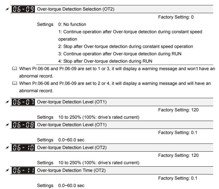
When the output current exceeds the over-torque detection level (Pr06-07 or Pr06-10) and also exceeds Pr06-08 or Pr06-11, the over torque detection will follow the setting of Pr06-06 and Pr06-09.
