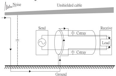
5. When excessive pulse modulated currents pass through an un-grounded AC drive cable, it acts as an antenna and creates radiated interference.
