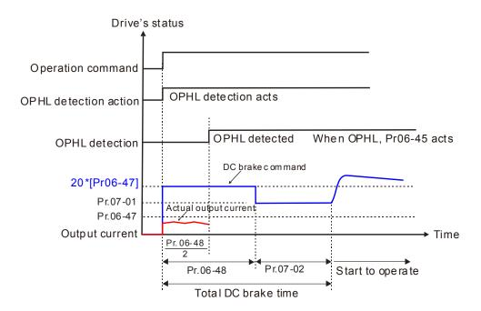
□ Status 4: Motor drive is in stop; Pr06-48≠0; Pr07-02=0
