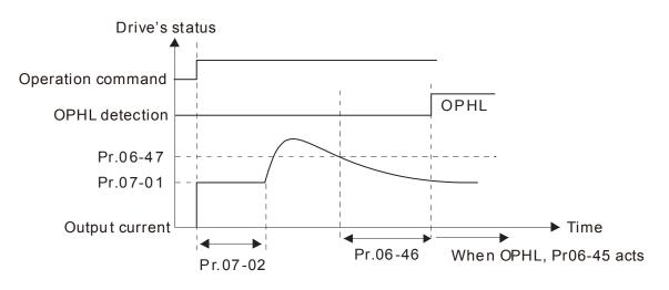
Status 3: Motor drive is in stop; Pr06-48 $\neq$ 0 ; Pr07-02 $\neq$ 0
