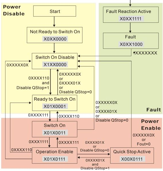
Set command 6040 =0xE, then set another command 6040 =0xF. Then the motor drive can be switched to Operation Enable. The Index 605A decides the dashed line of Operation Enable when the control mode changes from Quick Stop Active. (When the setting value is 1~3, this dashed line is active. But when the setting value of 605A is not 1~3, once he motor derive is switched to Quick Stop Active, it will not be able to switch back to Operation Enable.)
