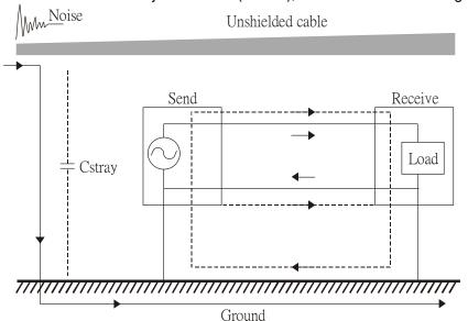
2. Common-mode noise in the power cable is transmitted through the stray capacitance and coupled into the adjacent signal cable, as shown in Figure 2. Several methods can be applied to reduce the effect of this common-mode noise; for example, shield the power cable and/or the signal cables, separate the power and signal cables, take the input and output side of the signal cable and twist them together to balance out the stray capacitance, let power cables and signal cables cross at 90°, etc.
