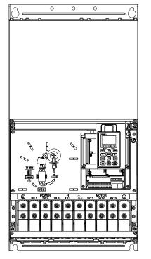
Main circuit terminals: R/L1, S/L2, T/L3, U/T1, V/T2, W/T3, +1/DC+, -/DC-
