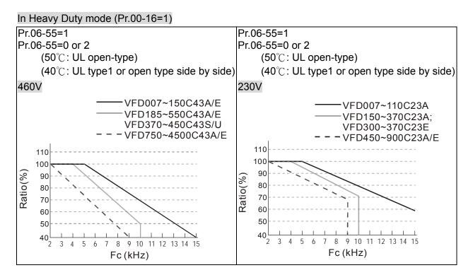
Ambient Temperature derating Curve for General Control Model
