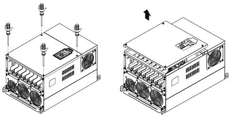
2. Fasten the 6 screws shown in the following figure and place the cover back to the original position. Screw torque: 24~26kg-cm (20.8~22.6lb-in).
