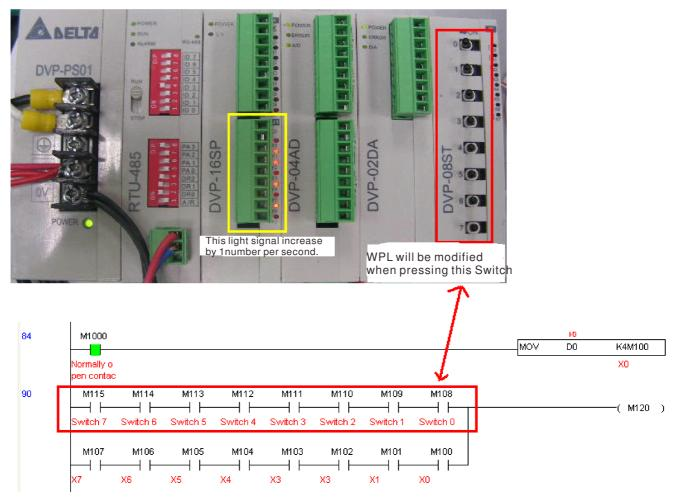
AD DA testing: It can be discovered that D200 and D201 are roughly twice the D300, and continue to increase progressively. For their part, the D202 and D203 are roughly twice the D301, and continue to decrease progressively.
