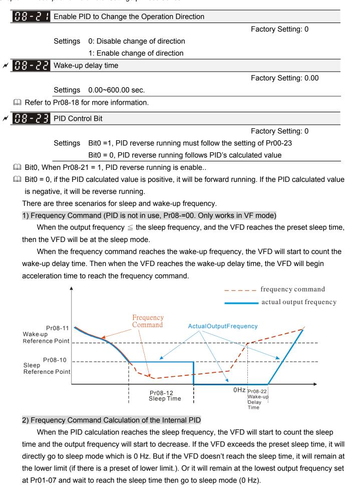
When the calculated frequency command reaches the wake-up frequency, the VFD will start to count the wake-up delay time. Once reaching the wake-up delay time, the VFD will start the acceleration time to reach the PID frequency command.
