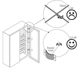
This is why a thick short ground wire must be implemented for connecting to the common grounding path or the ground busbar. Especially when a controller (e.g. PLC) is connected to an AC motor drive, it must be grounded by a short and thick conducting wire. It is suggested to use a flat braided conductor (ex: metal mesh) with a lower impedance at high frequencies.
