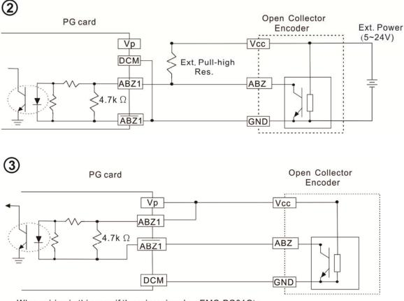
When wiring in this way, if there is a signal on EMC-PG010's A1, B1 and Z1, LED lights is OFF.
