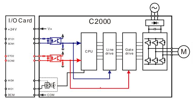
20-3-2 In the figure below, the factory setting for +24V-STO1-STO2 and SCM1-SCM2-DCM is short circuit:
