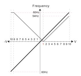
Pr.00-21=0 (Dgital keypad control and d run in FWD direction) Pr.03-05 Analog Positive Voltage Input Bias (AUI) = 10% Pr.03-07~03-09 (Positive/Negative Bias Mode) 0: No bias
