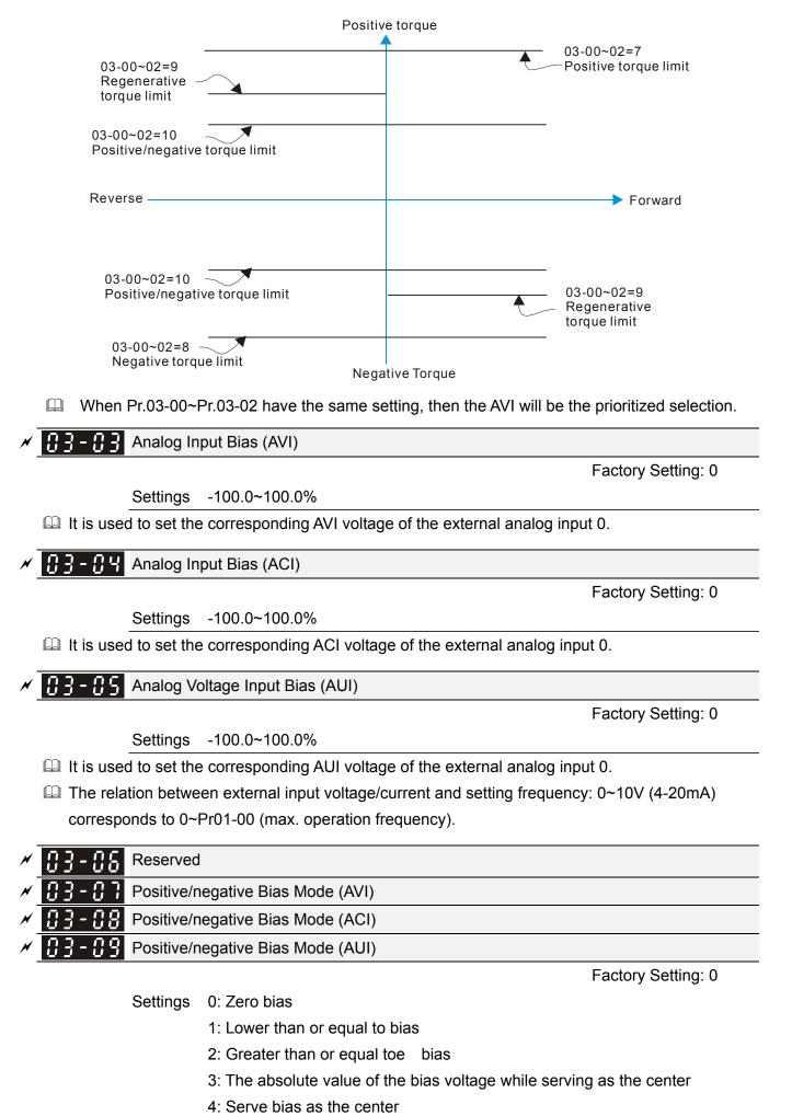
In a noisy environment, it is advantageous to use negative bias to provide a noise margin. It is recommended NOT to use less than 1V to set the operation frequency.
