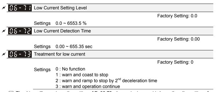
The drive will operate as the setting of Pr.06-73 when output current is lower than the setting of Pr.06-71 and when low current continues for a period longer than the setting of Pr.06-72. This parameter can also be used with external multi-function output terminal 44 (MO44) for low current output.
