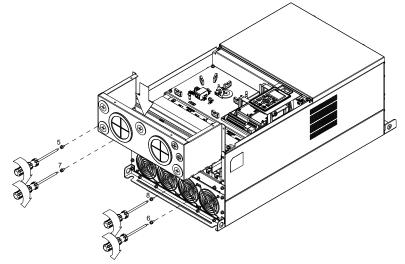
Install the conduit box by fasten all the screws shown in the following figure Screw 9~12 torque: 12~15kg-cm (10.4~13.6lb-in) Screw 13~16 torque: 24~26kg-cm (20.8~22.6lb-in)
